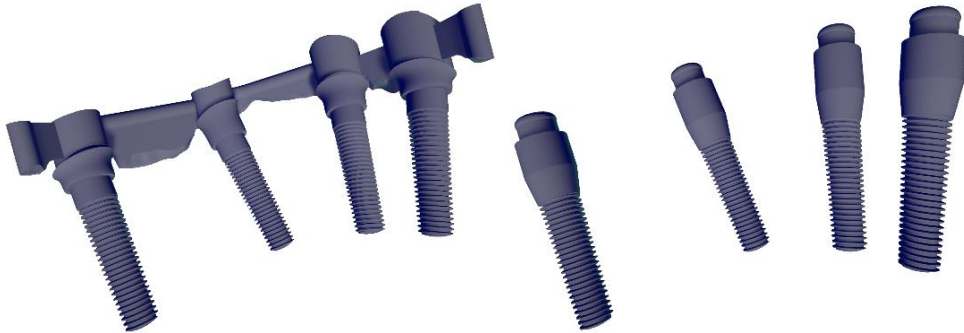
Fig. 3 Left—The splinted design chosen for analysis, right—the unsplinted locator design.
