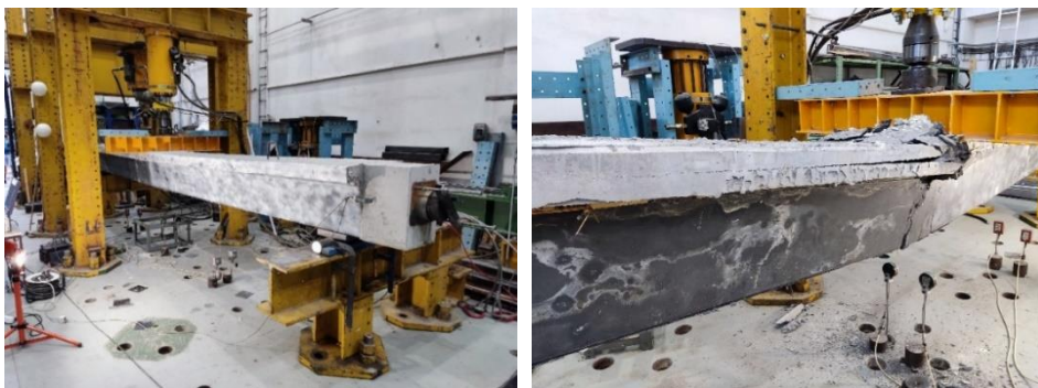
Fig. 2 Beam loading and the failure.
