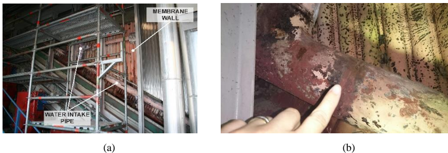
Fig. 2 (a) Membrane wall and water intake pipe, (b) cracks of welds on the water intake pipe.
