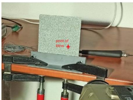
Fig. 2 Laying of the analyzed steel plate and the excitation point.
