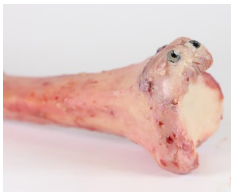
Fig. 3 Bone specimen with implanted screws.
