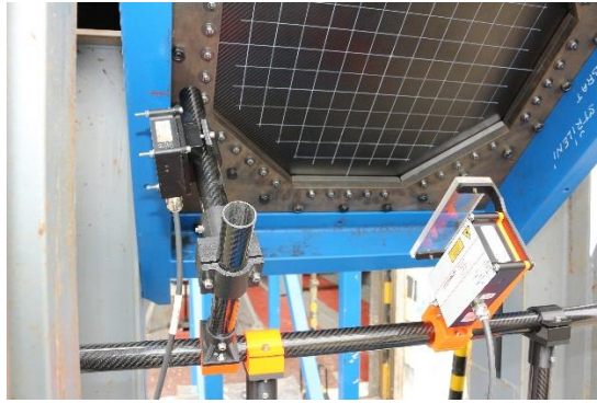
Fig. 5 Displacement measurement during the bird strike test.
