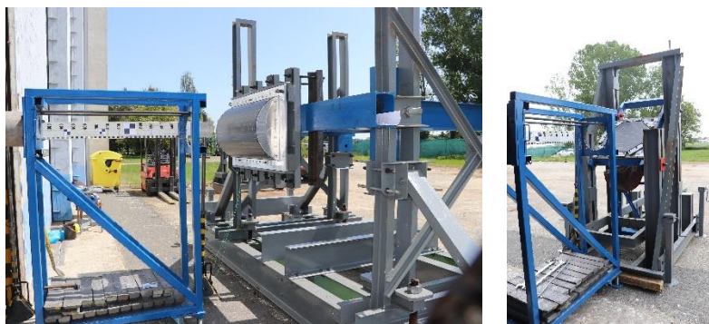
Fig. 4 VZLU test rigs to attached of curved (left) and flat (right) test specimen for bird strike tests.
