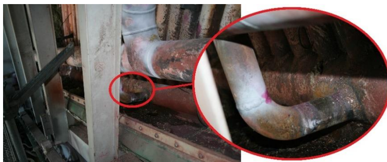
Fig. 7 Location of the sampling from the damaged piping system.
