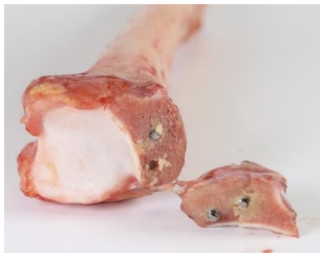
Fig. 4 Final destruction of a magnesium implant.
