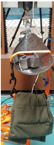
Fig. 2 Paddle during the laboratory loading.
