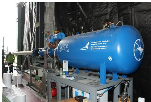
Fig. 2 VZLU air gun for bird strike tests.
