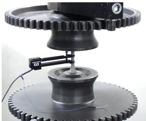
Fig. 3 Round static specimen test set-up – detail with an attached extensometer.
