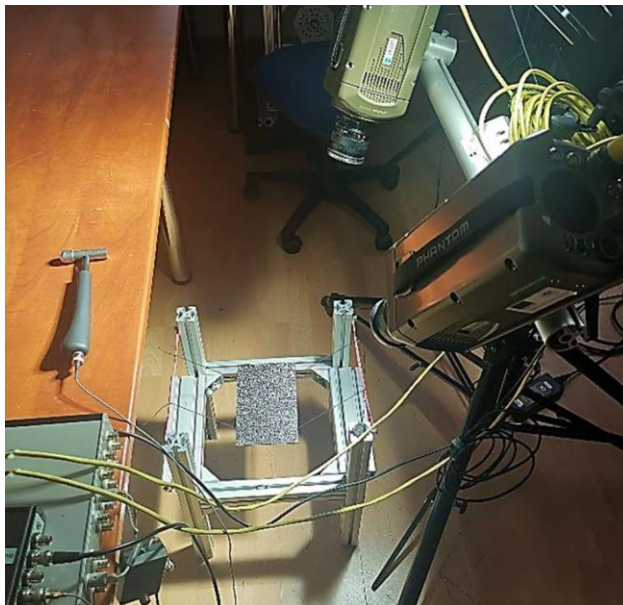
Fig. 4 Experimental configuration for measuring modal parameters of a composite plate.
