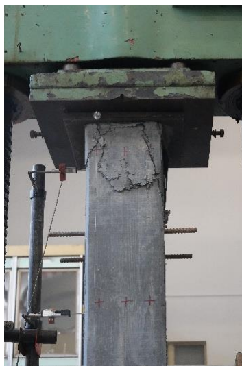
Fig. 5 Failure of the composite column.
