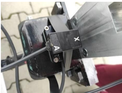
Fig. 9 Measurement point for acceleration in three axes.
