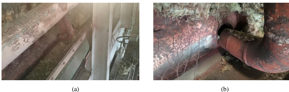
Fig. 3 Weld failure of the water intake pipe: (a) general view, (b) detailed view.
